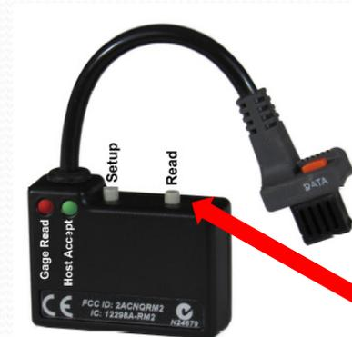
Mobile Module Buttons and LEDs
