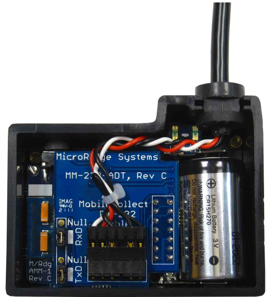
Gage Cable Connected to RS-232 Mobile Module with ATZB Radio
