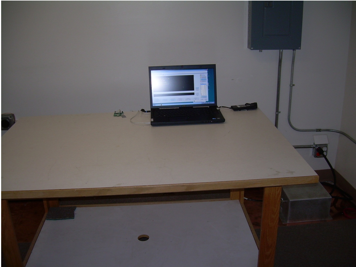
Photograph 5 – Front View Conducted Disturbance Worst Case Configuration
